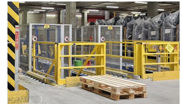
Automatic pallet check stations
